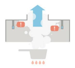
EcoAzur detects fumes, steam, or temperature change (or any of the three), and adjusts the ventilation system accordingly to maintain optimal air quality and maximize comfort.
