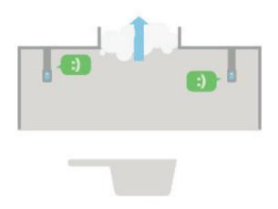
Once the temperatures return to normal within the hood and all fumes and vapor are gone, EcoAzur brings the exhaust and make-up air rates back to the preset level, or as low as 30% of full speed.
