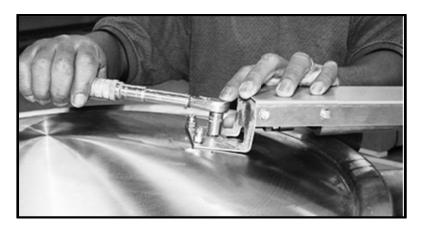
2.3 Ensure the kettle is tilted to the full upright position and then lower the cover over the kettle. Adjust the mounting bracket to align the cover over the kettle and then fully tighten the four nuts securing the actuator to the riser to a 10 ft/lb torque with a 1/4" open end or socket wrench.
