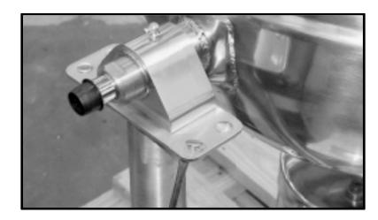
1.2 Remove the four hole plug caps in the left trunnion plate.
