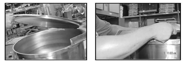
2.4 Install the handle spacers over the two studs at the front of the cover and apply thread locking compound to the ends of the two studs.
