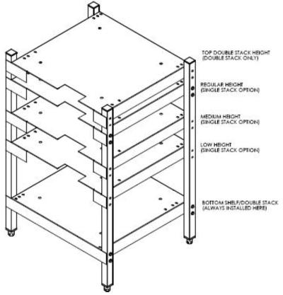
1.2 The above figure shows the shelf orientation for a single steamer, where the cutout in the lower shelf is turned to the back of the stand. For a double-stack stand, turn the shelf so the cut-out faces to the front.
