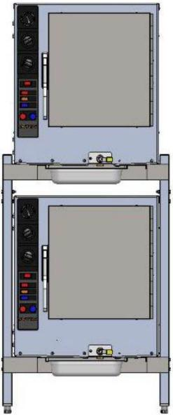
2.6. Note that the steamers mount directly to the shelves and the drain pans (standard  $12 \times 20 \times 4^{\circ}$  hotel pan) slide into the rails mounted underneath the shelves.
