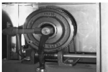
Liberally grease the wheel where it contacts the worm gear.
