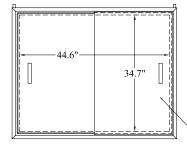
49" X 39" OPEN TOP REFRIG. 16GA S/S INTERIOR & EXTERIOR W/POLY SLIDING COVERS
