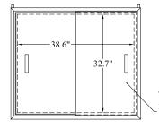
43" X 37" OPEN TOP REFRIG. 16GA S/S INTERIOR & EXTERIOR W/POLY SLIDING COVERS
